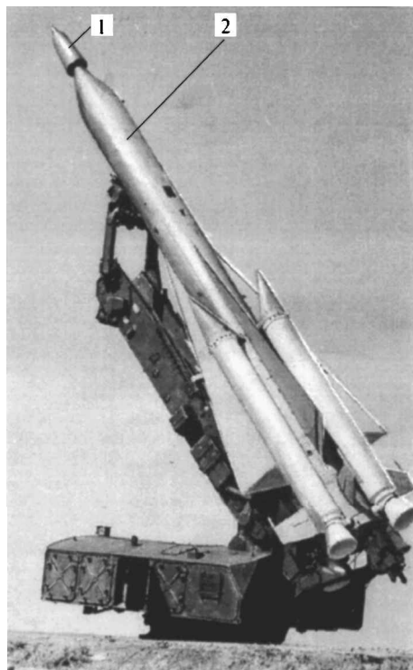
Fig. 1 Experimental DMSCRAM installed on rocket: 1, DMSCRAM; 2, "surface-air" rocket.
